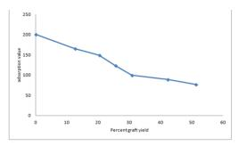
Figure. 8. The adsorption value of Hg2+ on poly (MAam)-pregelled starch graft copolymers having different graft yields.
