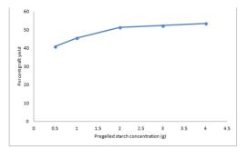
Figure. 4. Effect of pregelled starch concentration on percent grafting of poly (methacrylamide)-pregelled starch graft copolymer
