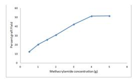
Figure. 2. Effect of methacrylamide concentration on percent grafting of poly (methacrylamide)-pregelled starch graft copolymer
