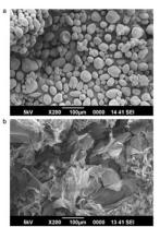
Figure. 10. SEM micrograph of (a) pregelled starch and (b) Poly (methacrylamide)-pregelled starch graft copolymer having 51.3 % graft yield.
