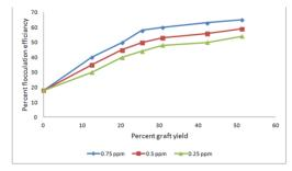
Figure. 7. Flocculation efficiency percent of pregelled starch and poly(MAam)-pregelled starch graft copolymers at different doses
