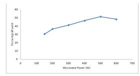
Figure. 3. Effect of microwave power on percent grafting of poly (methacrylamide)-pregelled starch graft copolymer
