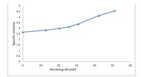
Figure. 5. Relation between percent graft yield of poly (methacrylamide)-pregelled starch graft copolymer and the specific viscosity
