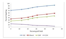
Figure. 6. Effect of percent grafting of poly (methacrylamide)-pregelled starch graft copolymer on swelling behavior using different solvent
